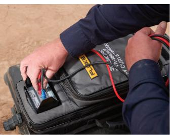
4 Fluke Corporation PVA-1500 Series PV Analyzer I-V Curve Tracer
