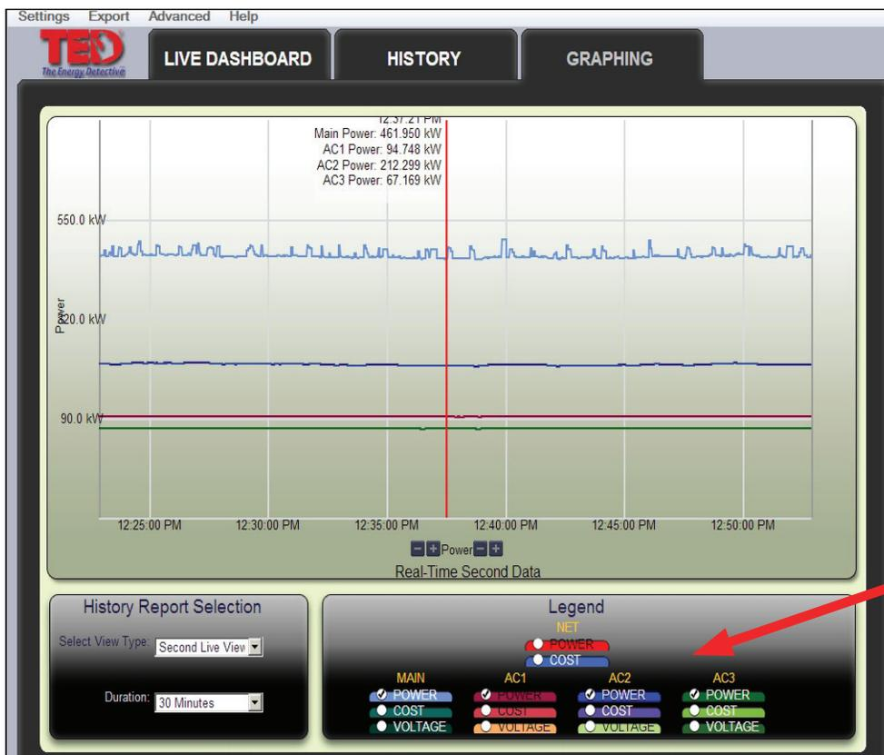
If more than 1 MTU is installed, each MTU may be graphed simply by checking the box under the name of the MTU.
