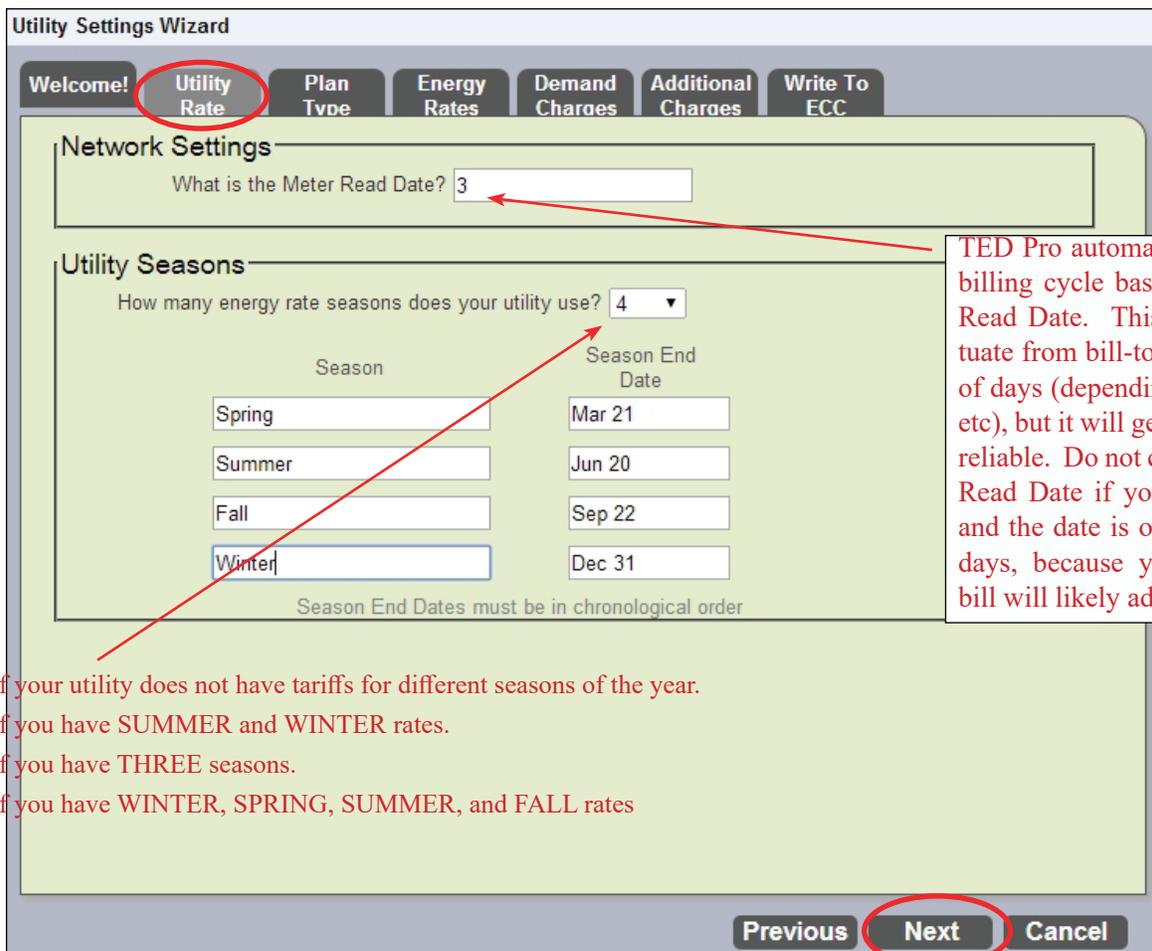
TED Pro automatically resets the billing cycle based on the Meter Read Date. This date may fluctuate from bill-to-bill by a couple of days (depending on weekends, etc), but it will generally be pretty reliable. Do not change the Meter Read Date if your bill comes in and the date is off by one or two days, because your next month bill will likely adjust for it.
