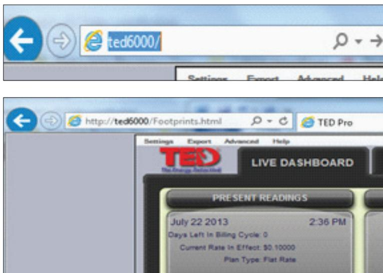
If your Browser does not load the Footprints page, you can access your router to determine the IP of the ECC and type the IP into the Browser address bar. You can also download the TED Installation Utility from the TED website (see the link below) and Run the installer. This 'installer' will locate the IP of your device. (If you do not have Internet access, see Appendix A of this guide.) Select your TED device when the installer locates it on your network and select *Launch in Browser*:
