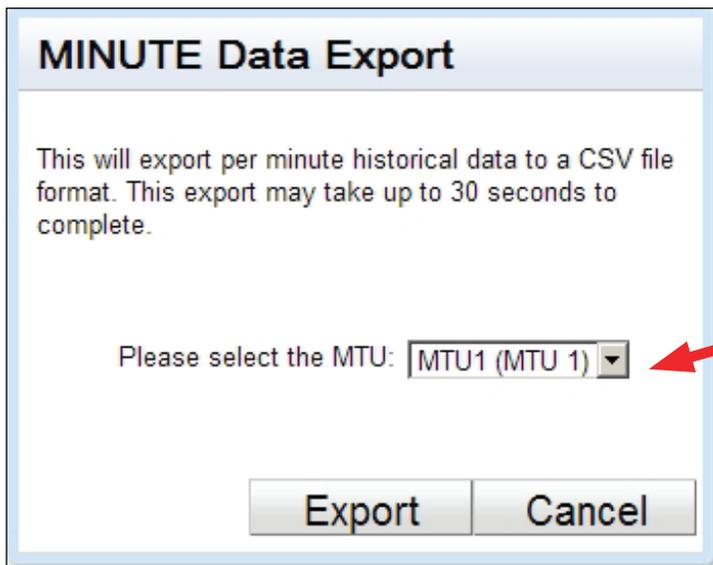
If you have multiple MTUs or a SOLAR/WIND installation, you can output the data for each MTU for analysis by clicking the drop-down.
