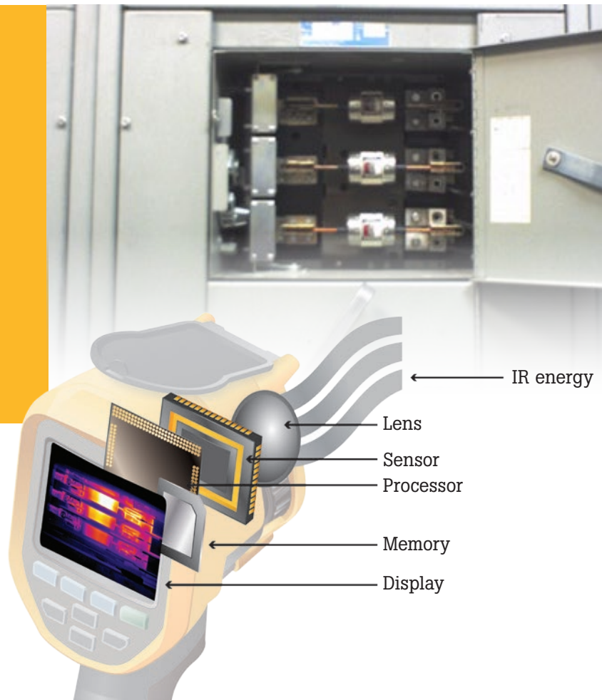
Figure 1. Anatomy of an infrared camera
