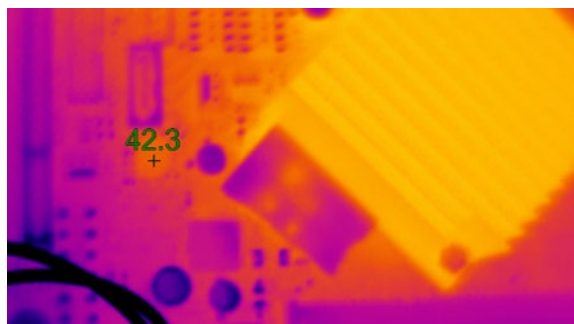
Figure 15. PCA running at 12V power supply
