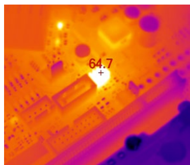
Figure 18. Operation with heatsink
