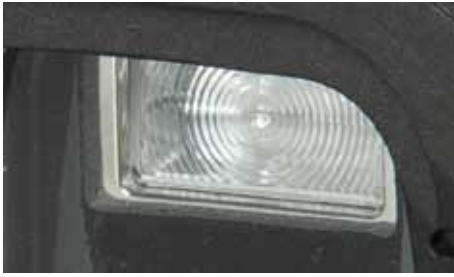
Onboard strobe flash for low light image capture
