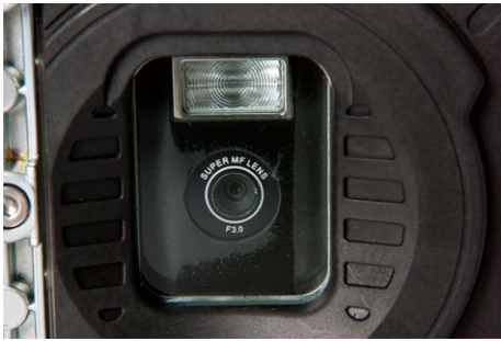
Strobe flash for low light imaging
