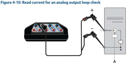
The Trex unit is connected to an analog output and is measuring current from the mA terminals. You can connect the Trex unit at various points on the current loop, including a junction box, device connection point, etc.
