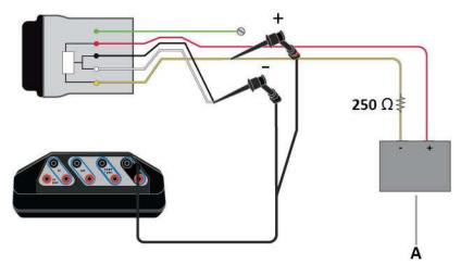
Connect the lead set to the yellow and white/black wires. The 250 Ohm resistor is not required, but it may be used to verify current.
