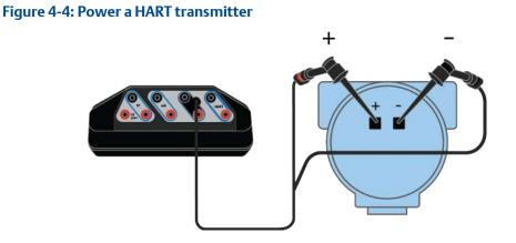
The Trex unit measures both voltage and current from the HART + pwr terminals. An internal 167 Ohm resistor is used when the Trex unit powers the device.
