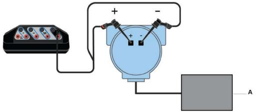
If you have a 250 Ohm resistor, you can insert it in between the device terminals and connect the lead set across the resistor. Otherwise, you can enable the internal resistor in the device connection wizard.
