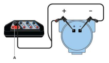
To power a FOUNDATION fieldbus device, the Trex unit needs the FOUNDATION fieldbus Power Plug. When the Trex unit powers a device, it also provides two terminators and a power conditioner.
