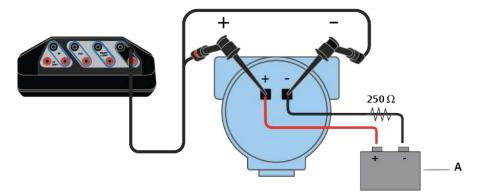
If the transmitter is at address zero, the Trex unit may automatically detect and connect to the device without any prompts from the device connection wizard.
