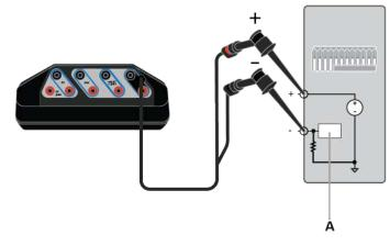
The Trex unit controls current from the HART terminals, which simulates a transmitter. The Trex unit controls current the same way as a transmitter controls current. The Trex unit is connected to the analog input (AI) channel.
