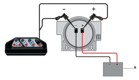
The Trex unit measures voltage from the HART terminals. Voltage measurements can be taken at various points to identify voltage drops along the loop.
