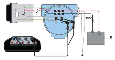
Figure 3-20: Communicate with the THUM adapter attached to a powered HART transmitter
