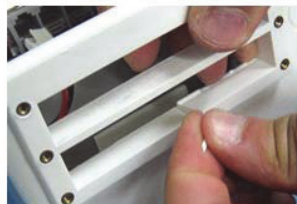
Removing Residual Material
