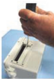
Opening Secondary Cable Slot
