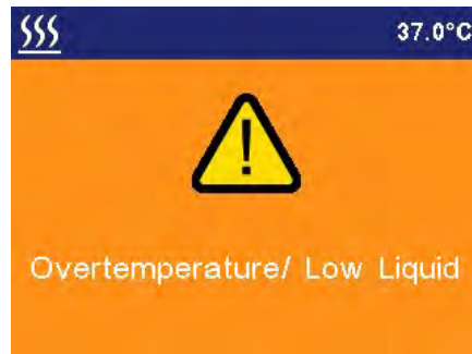
Example fault screen
