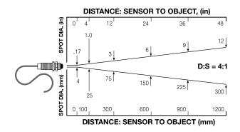
D:S is the optical resolution expressed as a ratio of the distance to the resolution spot divided by the diameter of the spot.
