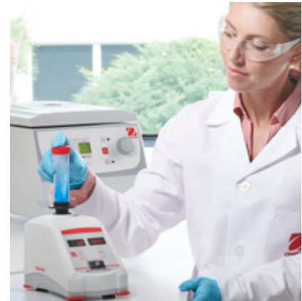
Vortex Mixers used to agitate or re-suspend samples
