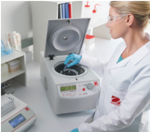
Centrifuges used to isolate desired contents of sample
