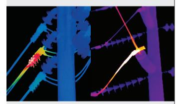
Thermal imaging surveys can give you a full picture of potential problems so you can prevent failures before they occur
